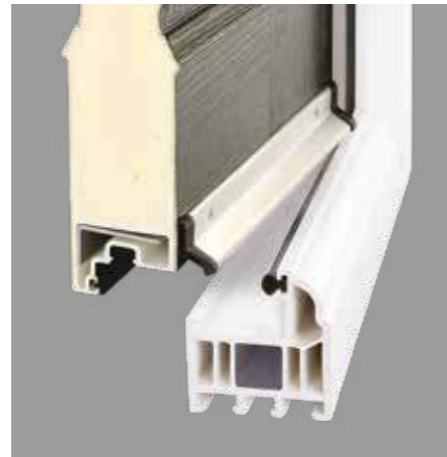
uPVC Low Frame Threshold Distance from bottom of door leaf to bottom of threshold 27mm
